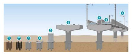
Figure 1. Sequential steps of installing rail bridge.
