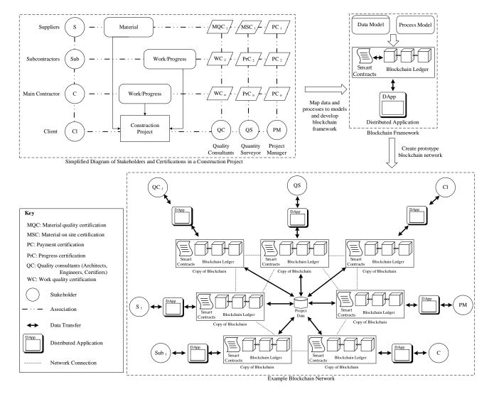
Figure 2. Conceptual model for blockchain-based work and payment certification
