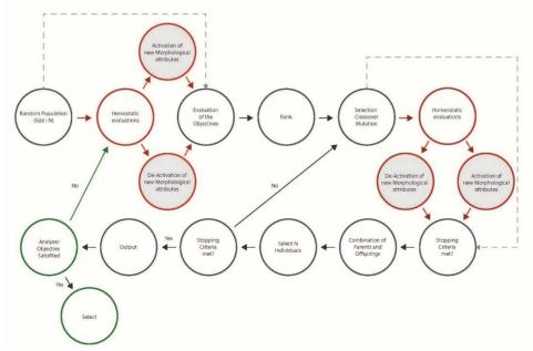
**Figure 2.** The modified evolutionary simulation workflow with two secondary evaluation mechanisms. The red squares show the modified stages. The green square shows the added step on the application of evolutionary simulation.
