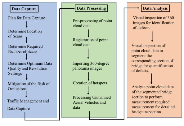
Figure 1. The proposed digital bridge examination process
