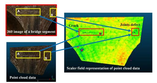
Figure 6. Detection of crack and joint defect.
