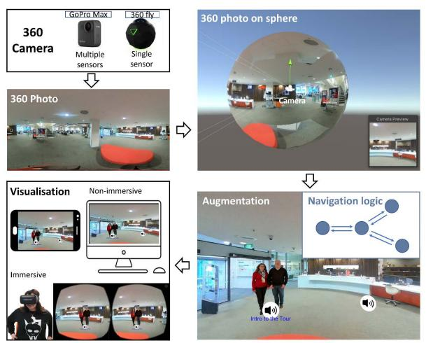
Figure 1. Prototyping steps to develop a VFT using 360 photos
