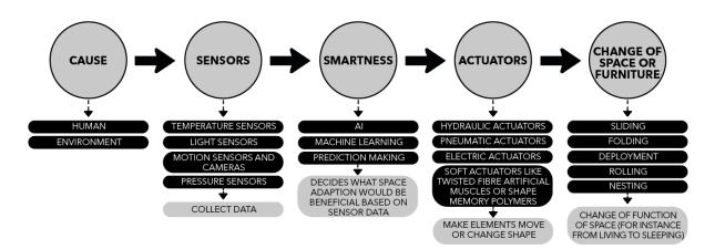
**Figure 3.** Technology for adaptive spaces Source: own graphic
