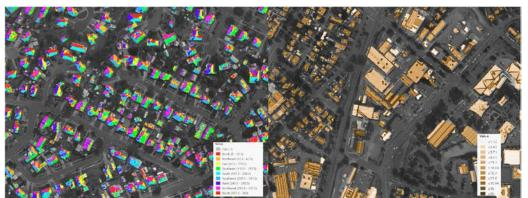
Figure 2. Geoprocessing outcomes of rooftop angular parameters (Left: Azimuth angle; Right: Tilt angle)
