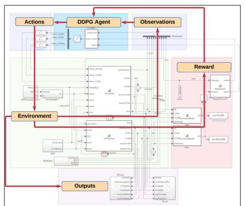
Figure 5. Simulink RL model built based on the MDP for VPP economic dispatch model
