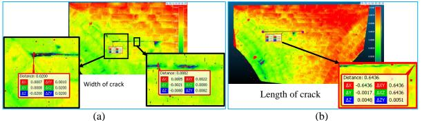
Figure 7. (a) measurement of the width of the crack, (b) measurement of the length of the crack.
