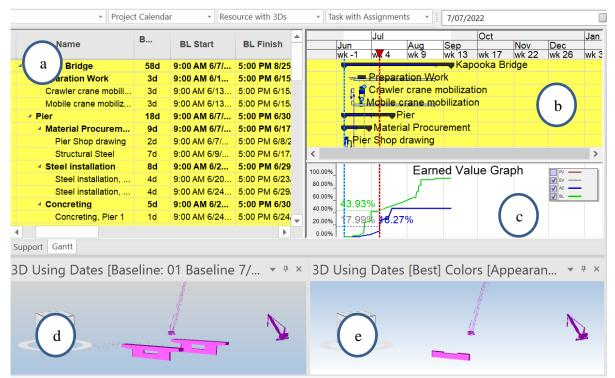
**Figure 3.** Interface for construction progress: (a) Schedule, (b) Gantt chart, (c) Earned Value Graph, (d) Planned 3D model, and (e) Actual progress 3D model.
