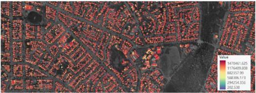
Figure 3. Rooftop solar irradiation potential raster
