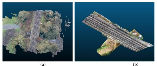
**Figure 5.** (a) captured data by UAV from the topside of a track, (b) image of combined UAV and TLS captured point cloud data.
