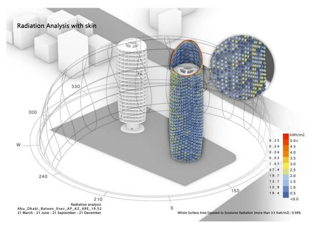
Figure 9. Radiation Analysis of the tower with the new optimised skin (after the simulation)
