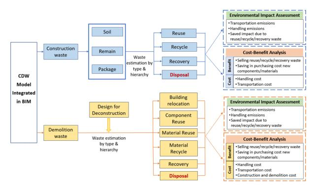
Figure 2. Conceptual framework for a decision support tool for designing out waste
