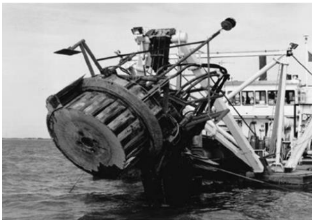
Figure 1: Environmental Disc Bottom Cutter Dredge
